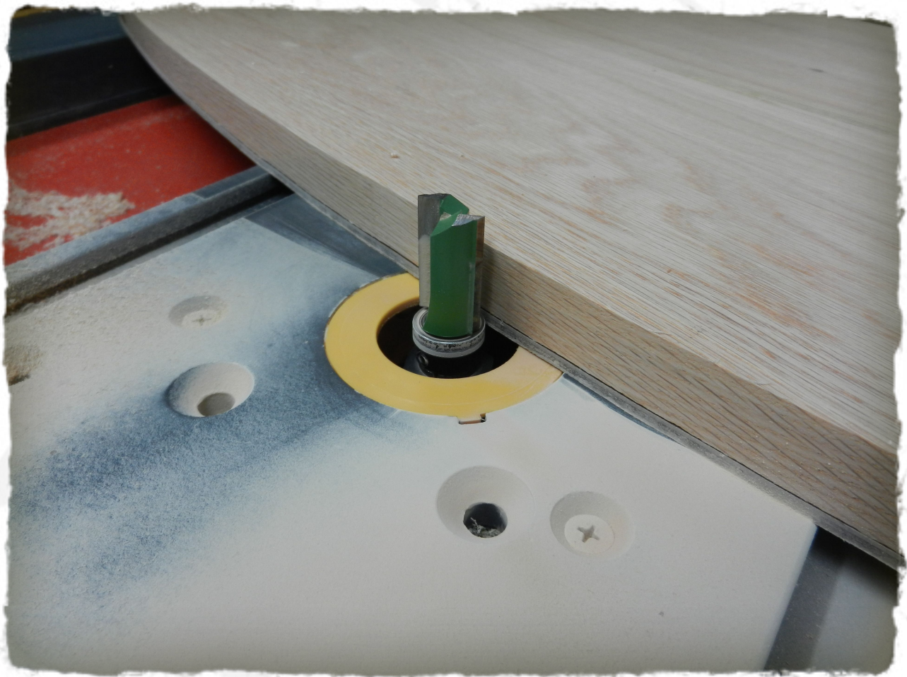
Using a template bit to cut the bow arc on the Shelf (E)
